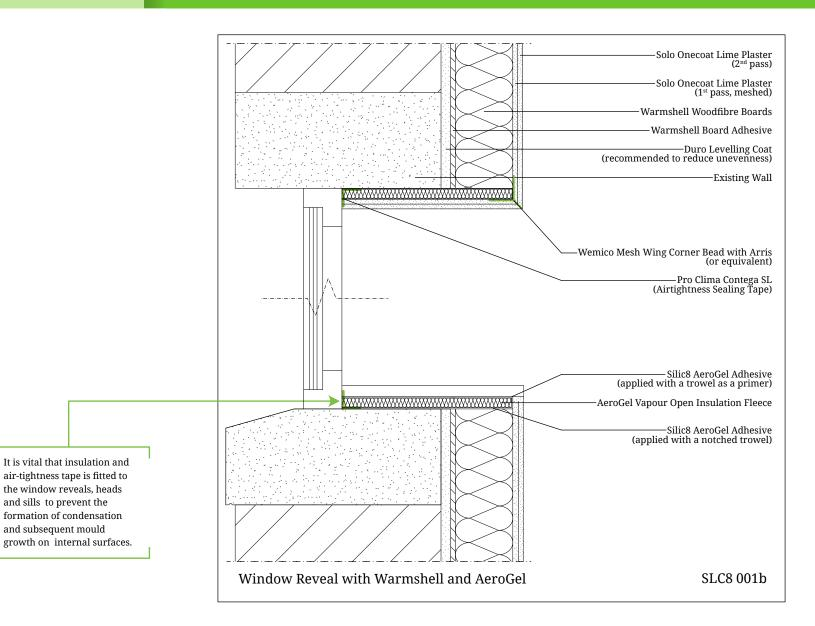
10mm of insulation in the reveals and head is more effective at saving energy than doubling the main insulation on the wall.
